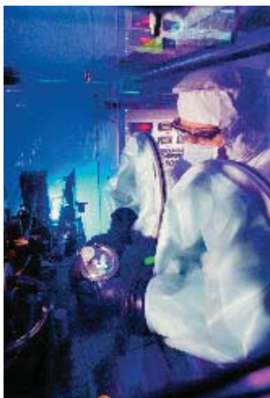
The Class III cabinet is defined as a ventilated glovebox.
