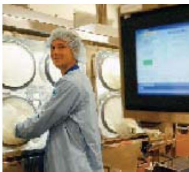
The glovebox is maintained under negative pressure.
