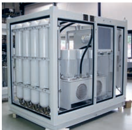
Hydraulic power unit
