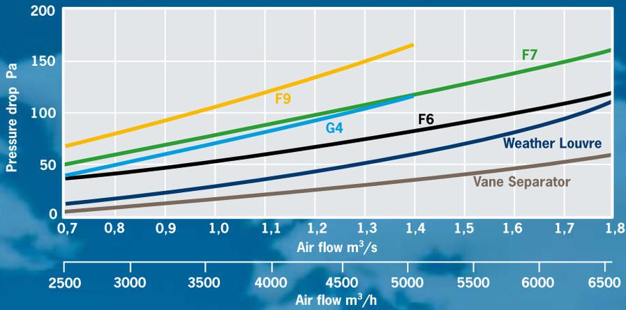
Pressure drop for clean filters, Wheater Louvre and Vane Separator.
