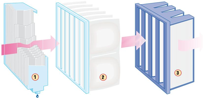
CamVane Droplet Separator or Weather Hood
