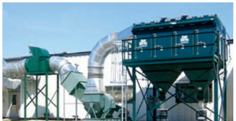
GS48 on wood finish sanding
