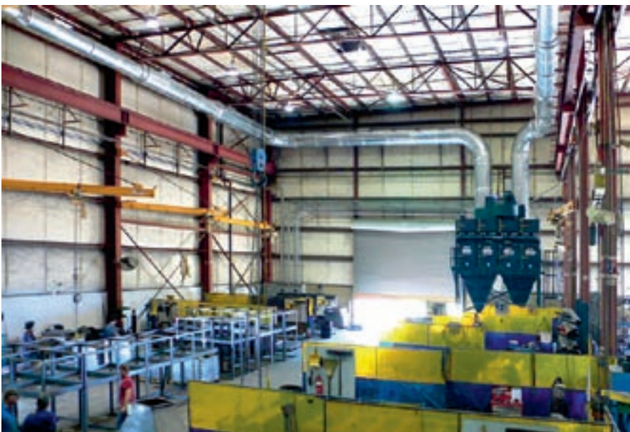
GS48 on weld fumes with integral HEPA
