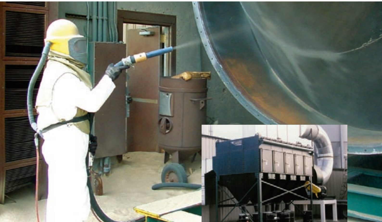
GS60 on windmill tower grit blasting
