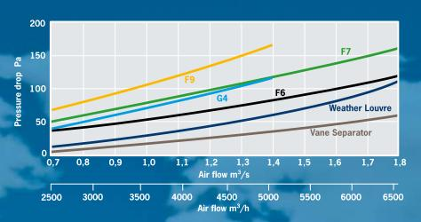
Pressure drop for clean filters, Wheater Louvre and Vane Separator.
