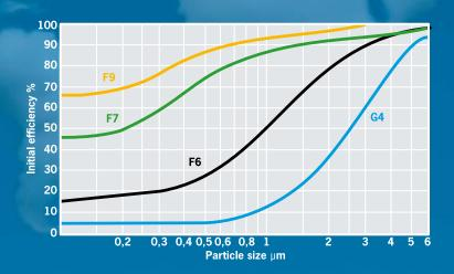
Particle arrestance for clean filters during tests in accordance with EUROVENT 4/9.
