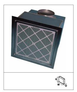
**Description:** Fully welded ducted filter module for HEPA or ULPA filter. Available with bubble-tight, guillotine or radial blade bowtie damper for precise airflow control. A test shroud is available for overall efficiency testing from the room side.
